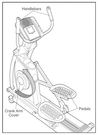
To dismount the elliptical exerciser, wait until the pedals come to a complete stop. Note: The elliptical exerciser does not have a free wheel; the pedals will continue to move until the flywheel stops. When the pedals are stationary, step off the higher pedal first. Then, step off the lower pedal.
